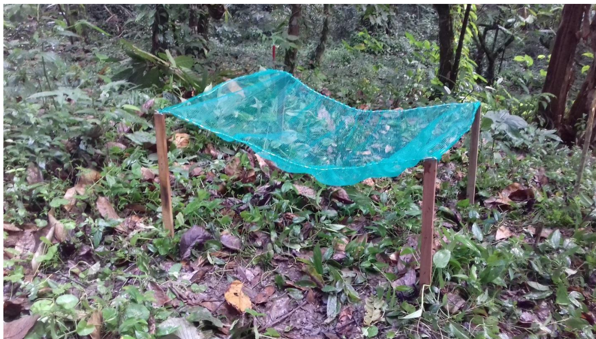
Figure 1. Photo of a seed collector installed in a cacao agroforestry sampled in south Bahia.
